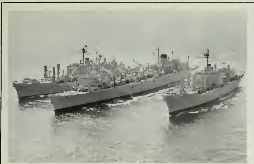
SUPPLY ADVANCEMENT —Latest word in underway replenishment is seen in this photo of three new supply ships. Fast combat support ship USS Sacramento (AOE 1) (center) combines jobs of fleet oiler, ammunition and refrigerated stores ships into one. USS Mars (AFS 1) (top) and USS Sylvania (AFS 2) are first of combat stores ships class, combining the functions of aviation, general and refrigerated stores ships.
